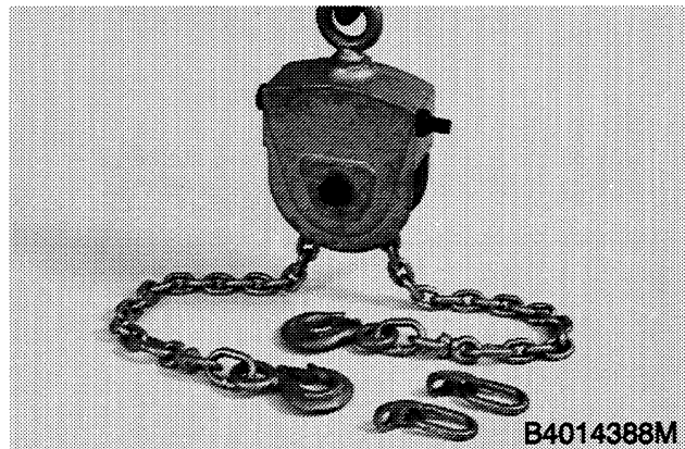
The lifting sling is used to remove and install the engine. The part number of the tool is CAS-10119. This tool is first used on page 2001-9.
