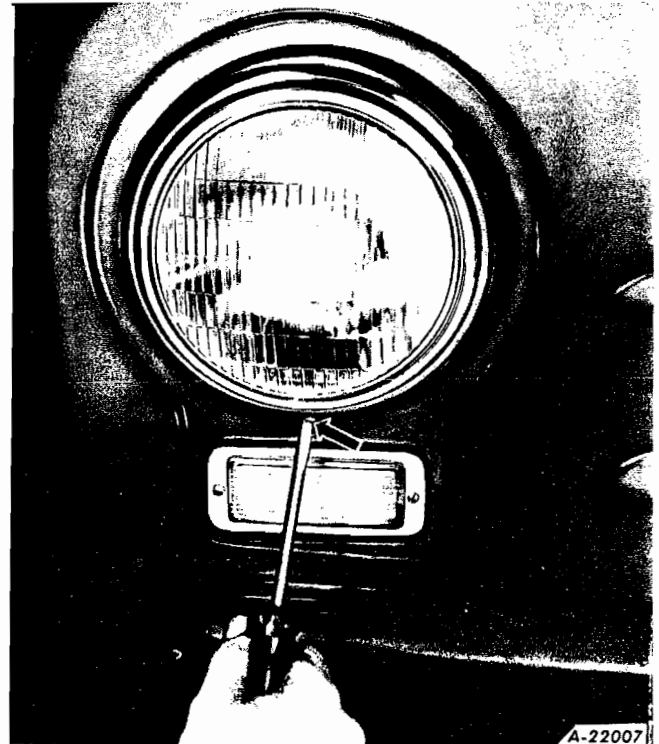
Fig. 1 - Removing headlight door.
